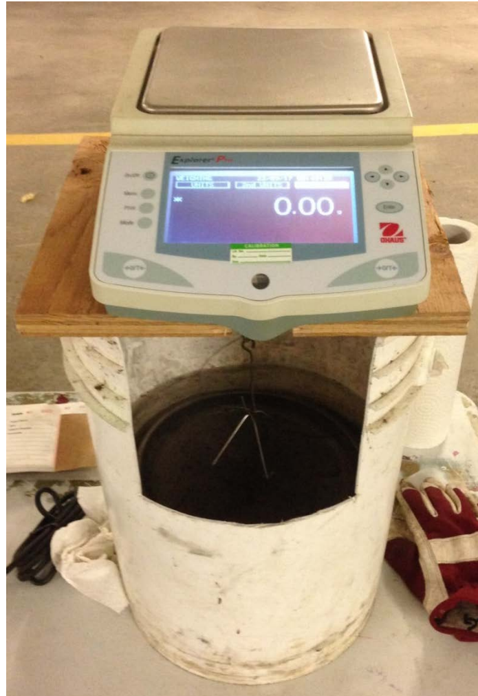
Figure 12-3 Balance scale and water bucket setup for measuring specific gravity of core (Source: Blind Creek, 2018)
