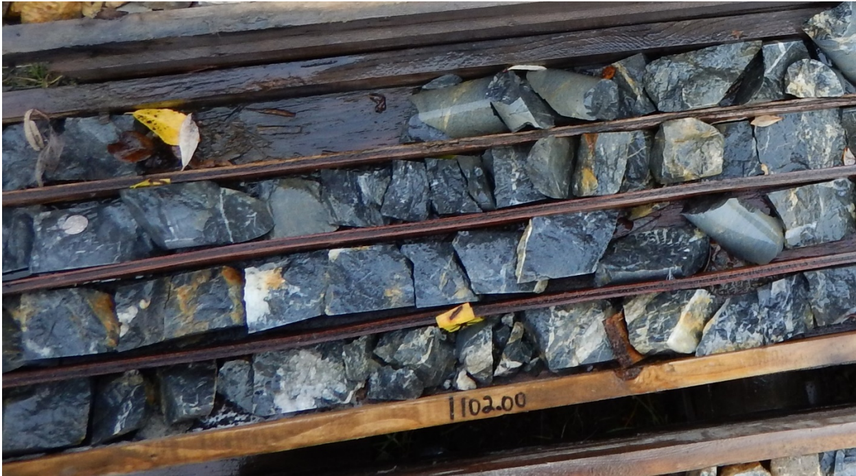
Figure 12-2 Typical competent drill core sampled for SG test work (Source: Blind Creek, 2018)
