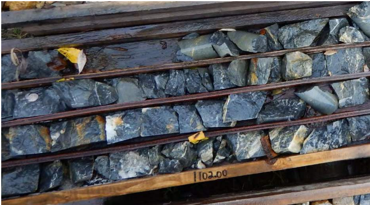
Figure 12-2 Typical competent drill core sampled for SG test work
